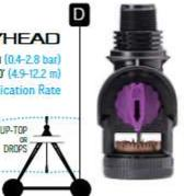
The **Sprayhead** is a fixed spray designed with future needs in mind. As irrigation requirements change throughout the season, the **Sprayhead** features a flip-over cap to change spray patterns. It's easily convertible to LEPA or other sprinkler types. 3000 Series (3TN nozzle) or 3030 Series (3NV nozzle).
