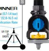
The **Spinner** utilizes a free-spinning action to produce a gentle, rain-like water pattern. Designed for more sensitive crops and soils, low instantaneous application rates and reduced droplet kinetic energy help maintain proper soil structure. 3000 Series (3TN nozzle) or 3030 Series (3NV nozzle).
